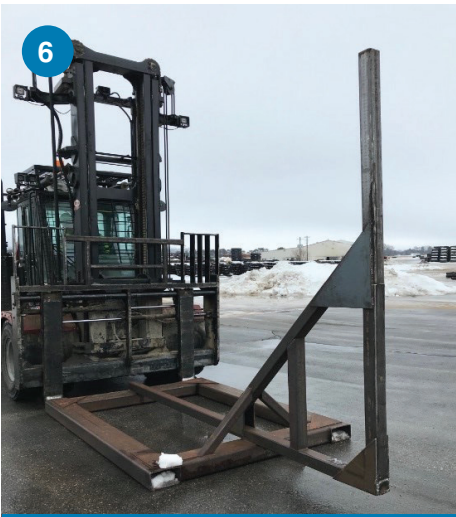
6 Example of pusher bar fabricated for forklift and used to brace packs during unloading
