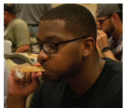
Titus Mills of Koppers tests the porosity of red oak by dipping one end in soap bubbles. Looks like this piece has no tyloses.
