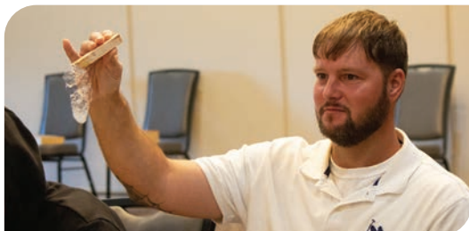
Dustin Roseberry of Stella-Jones shows off his red oak bubbles. No tyloses in red oak means that air passes through the wood to the bubble solution.
