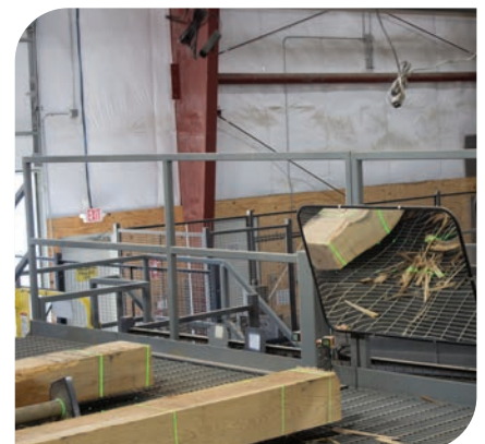
Ties from the grader's perspective. Within a few seconds the grader decides species and defects and sorts the ties accordingly. ▶
