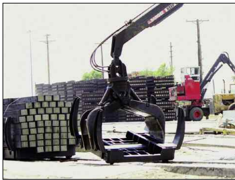
More from the Koppers plant. The tie unloader resetting a treating cylinder tram.
